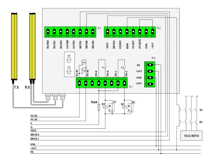
If not used the external contactors control, connect the EDM input to +24V of X2 connector.
