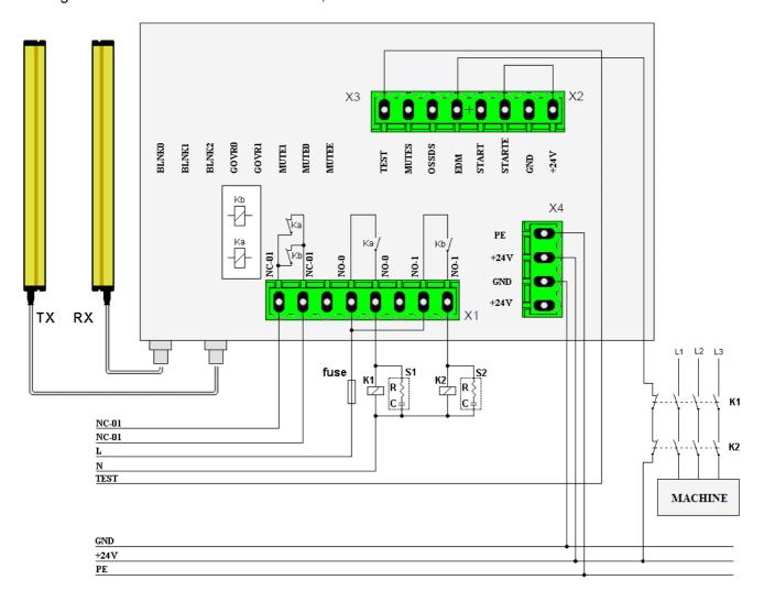
If not used the external contactors control, connect the EDM input to +24V of X2 connector.
