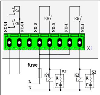
If the relays K1 and K2 do not have arc suppressors, we suggest to install the filters of the following value:
