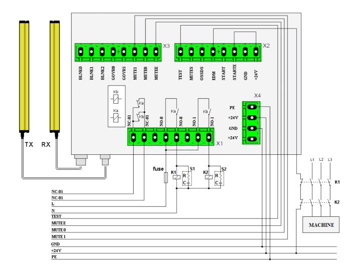
If not used the external contactors control, connect the EDM input to +24Vdc of X2 connector.
